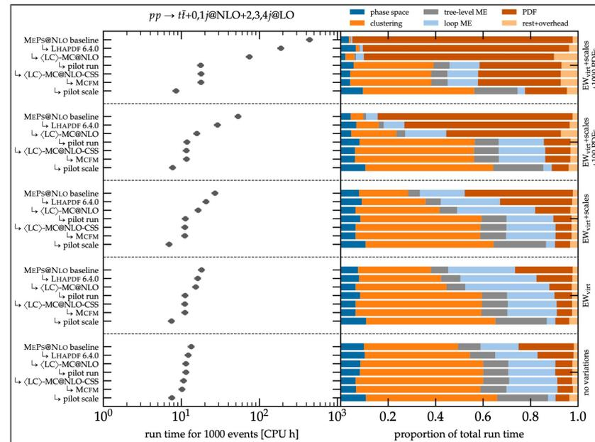
Very large speedups (**x2-78**) demonstrated when running ATLAS setup with >100 weights (EW, PDF,...) using *simplified pilot runs and fast PDFs*
